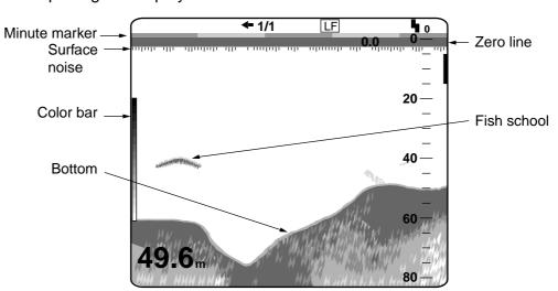
This section provides, using typical examples, the information necessary for interpreting the display.
